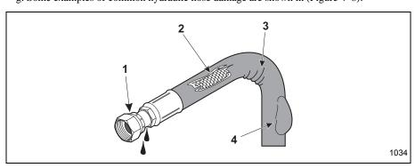
Figure 4-8 Hydraulic Hose Damage
